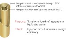
The compressor is subjected to a heavy load when compressing liquid refrigerant, and the result is lower operation efficiency. The addition of HIC supports refrigerant heat exchange at two different pressure levels. The heat-exchange process transforms the injected liquid refrigerant into a gas liquid state, thereby decreasing the load on the compressor during the compression process. **B** Injection Compressor
