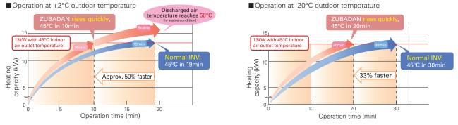
ZUBADAN Defrost Control and Faster Recovery from Defrost Operation Field Test Results: Office building in Asahikawa, Hokkaido, Japan
