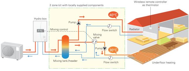
\*Items such as a mixing tank, mixing valve flow switch and pumps are not included and need to be purchased locally.
