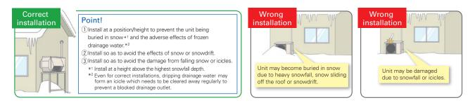
Use a stand to add sufficient height to protect the unit heat exchanger from snow and prevent icicles forming during defrost operation.
