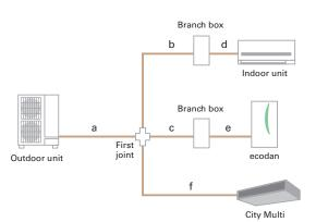
\*When an ecodan is connected, the maximum piping length is 150m.
