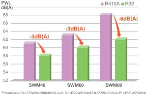
\*Compared SUZ-SWM40/60/80VA with SUHZ-SW45VA/PUHZ-SW50VKA/PUHZ-SW75VHA \*Rated condition (According to EN12102)
