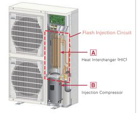
The ZUBADAN Series is equipped with Mitsubishi Electric's original Flash Injection Circuit, which is comprised of a bypass circuit and heat interchanger (HIC). The HIC transforms rerouted liquid refrigerant into a gas-liquid state to lower compression load. This process ensures excellent heating performance even when the outdoor temperature drops very low.
